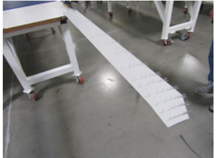
The HVAB blade with primer coat shows pressure sensors before trimming. The blade is a bonded assembly with integrated sensors and conductors. (ATI photo)
